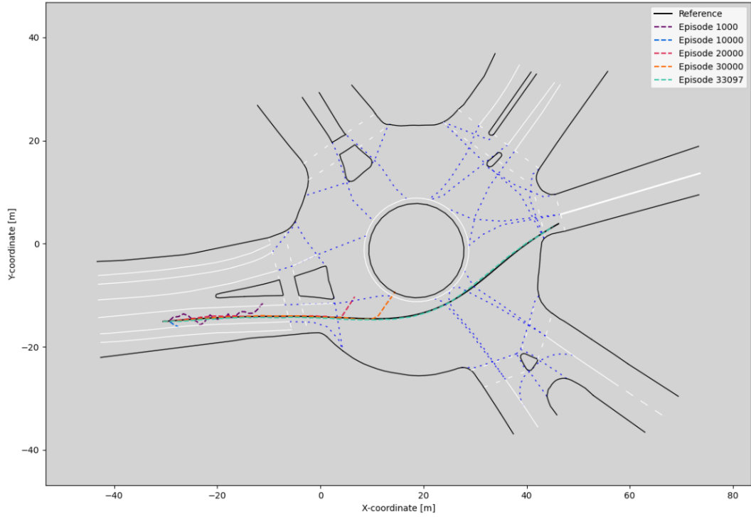
Figure 4.5: Selected trajectories from the training cycle with the settings in Tab. 4.6. The according episode can be seen in the legend.
